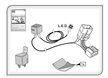
C2 control unit for vehicles with an 8 pole flasher relay.
